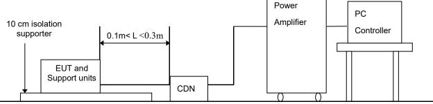
For the actual test configuration, please refer to the related item – Photographs of the Test Configuration Note: 1) The EUT is setup 0.1 m above Ground Reference Plane
